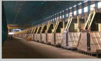
Aluminum smelter projects require fabrication and installation of aluminum bus bar network around their electrolytic pot cells. The fabrication job is carried out at a site machine shop. The job involves cutting various heavy rectangular section (ranging from 400 X 200 mm to 200 X 120 mm) by circular saw, band saw.
